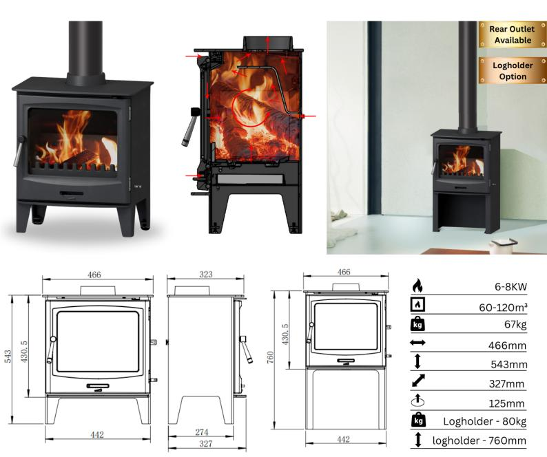
The LSO7 stands out as a compact yet efficient heating solution. Its advanced design incorporates a preheated air intake and multiple intakes through the ashpan and back of the unit, ensuring thorough combustion and effective heat distribution. The secondary air, heated at the top of the unit, flows over the viewing glass, maintaining a clear view of the flames.
